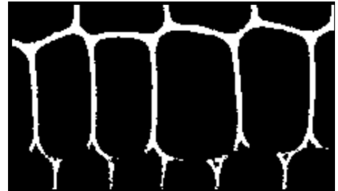
Threshold too high
